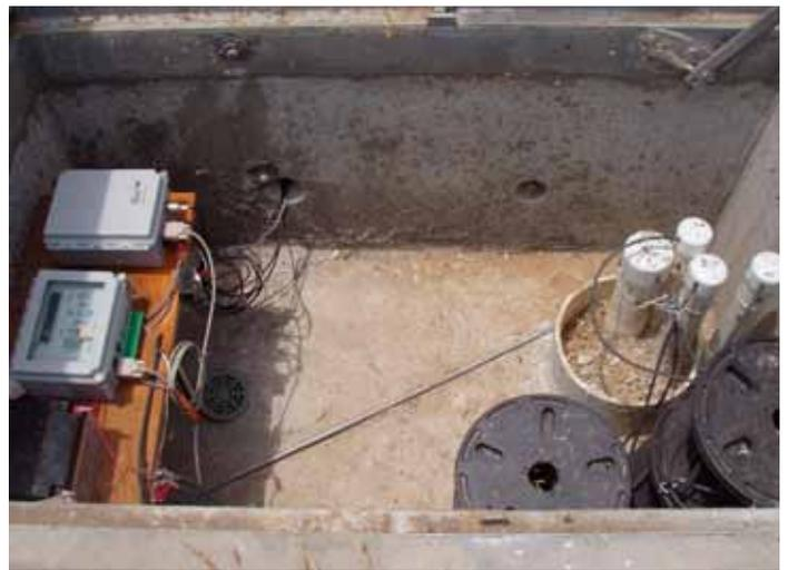
Figure 3D. Inside of a typical vault showing piezometers, transducer wires, data logger, and satellite link. Real-time data is provided via the Internet.
