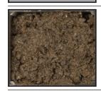
1,000-1,020: Gravelly sand (gS); very fine to very coarse sand with granules to small pebbles and minor silt; very angular to subangular; very poorly to poorly sorted; light olive brown (2.5Y 5/3); calcareous.
