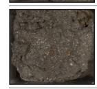
300-310: Sand (S); very fine sand with minor silt; well sorted; subangular to subrounded; very dark grayish brown (2.5Y 3/2).
