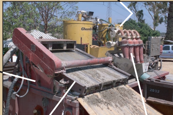
The desilter cones or desander separate the finer sands from drilling mud.
