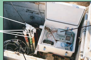
Wires attached to two advanced tensiometers and seven heat dissipation probes
