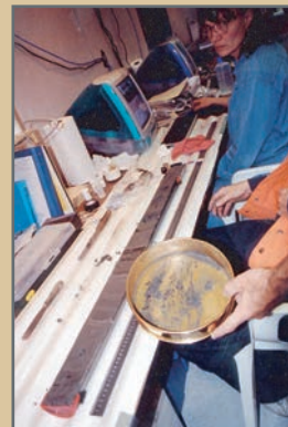
Liner is cut and core is described
