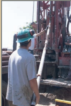
5-foot barrel attached to 5-foot spring retract
