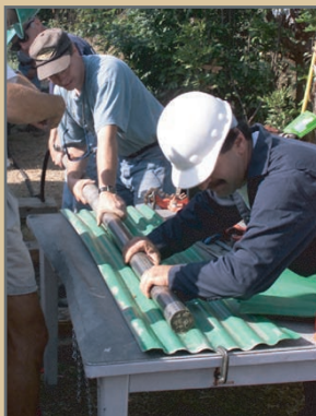
Extraction of liner containing core material
