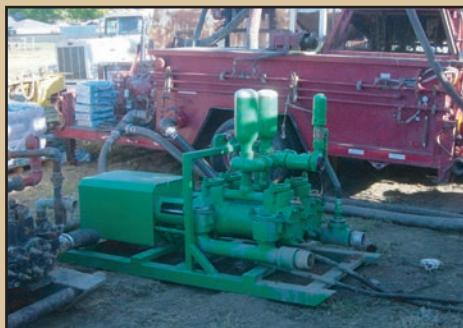
Dual positive displacement (piston) mud pumps force the drilling fluid down the borehole when the rig's centrifugal pump is over pressured. These pumps are used at deeper depths.
