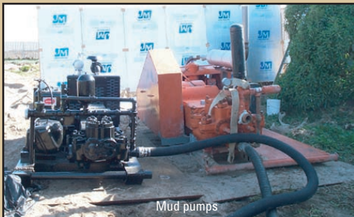
Dual positive displacement (piston) mud pumps force the drilling fluid down the borehole when the rig's centrifugal pump is over pressured. These pumps are used at deeper depths.
