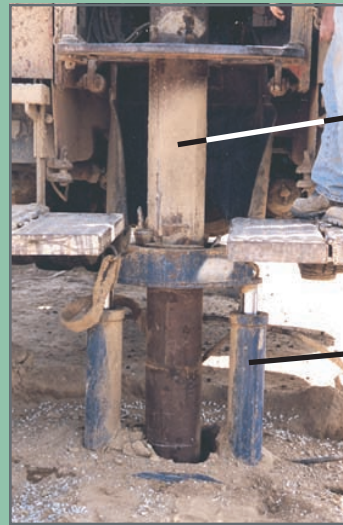
8-inch threaded casing (6-inch is also available for use with this system)
