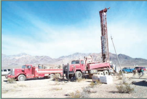
Drilling site using air-hammer drilling method
