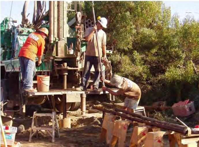
Figure 3C. Core samples are taken from selected depths using a wire-line device. Cores help correlate geologic layers.
