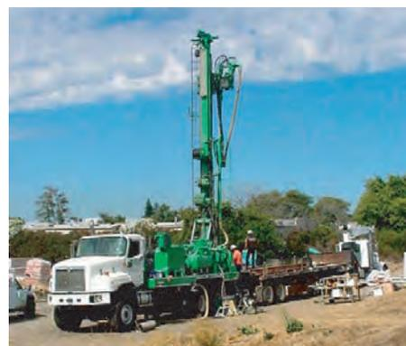
**Figure 2.** Typical drill rig used to construct a multiple-depth monitoring well.
